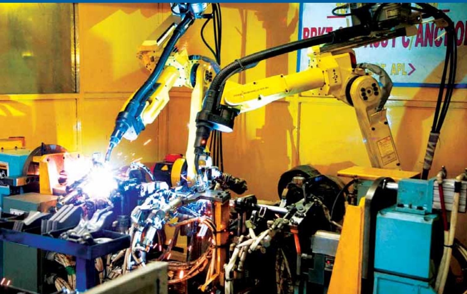
Precision robotic MIG welding of bracket cross anchor assembly
