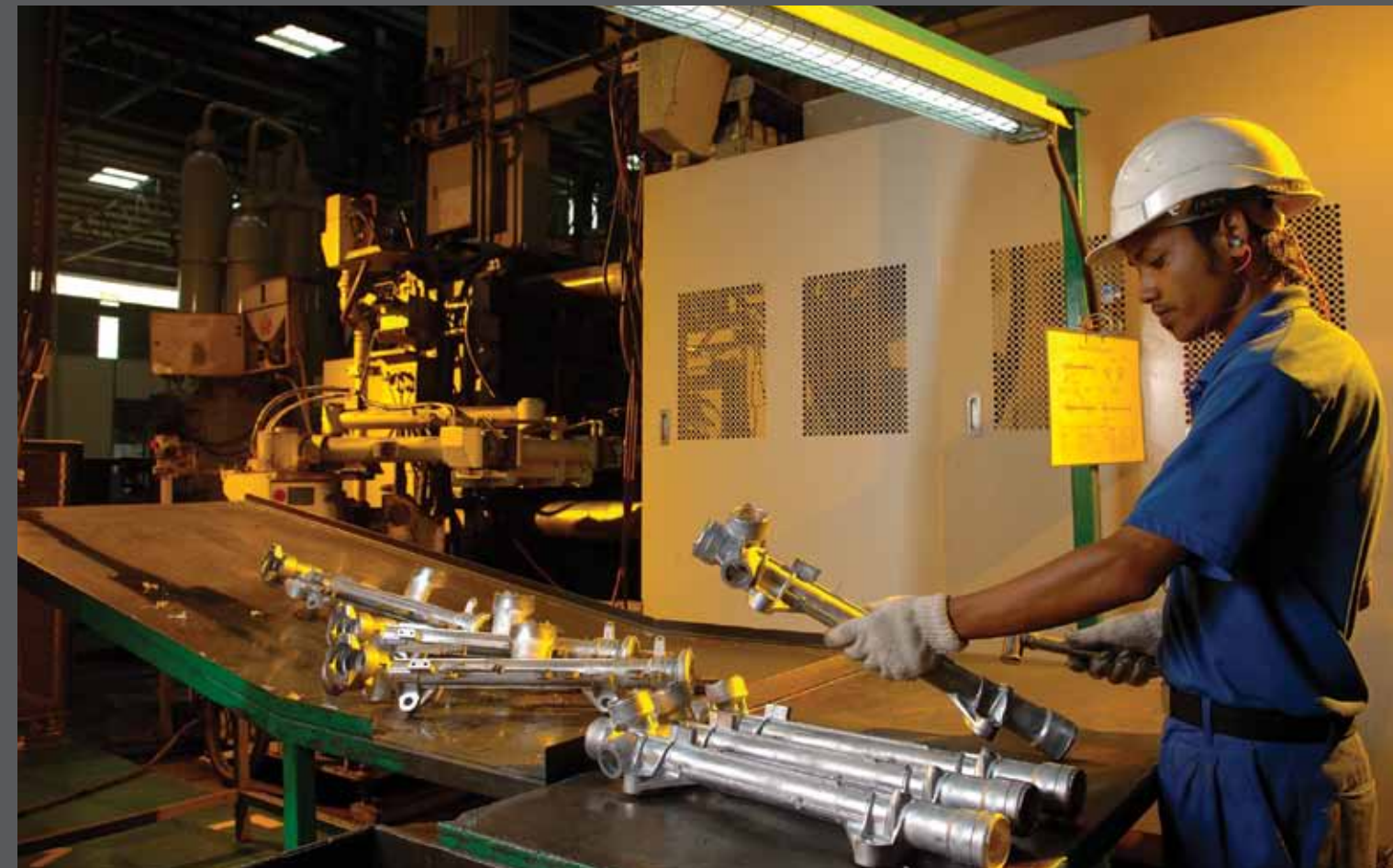
Aluminium diecasting of Steering Housing
