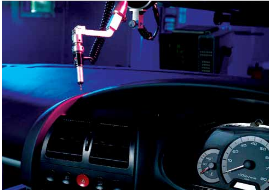
Coordinate measurement of Instrument Panel Assembly
